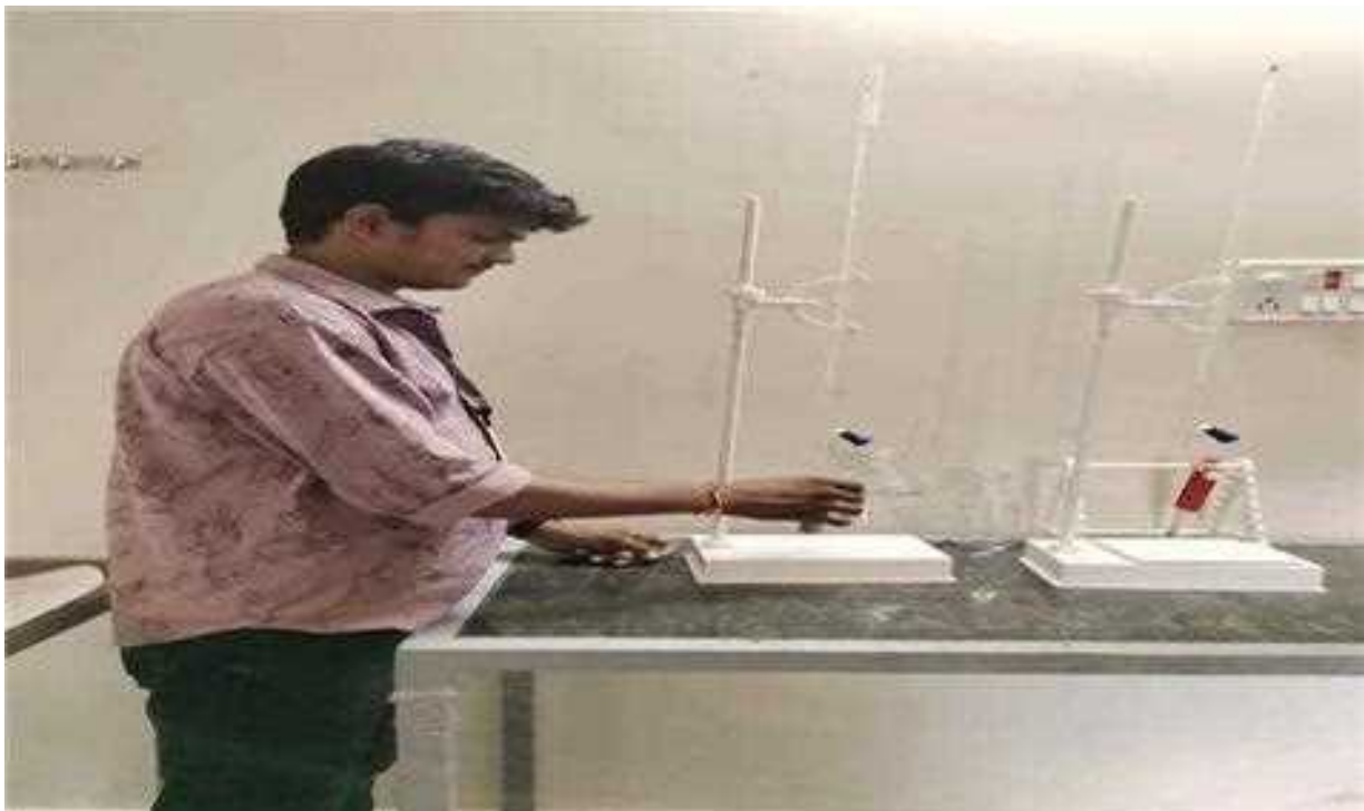
Fig 6 :- Determination of alkalinity and hardness through titration by adding indicators
