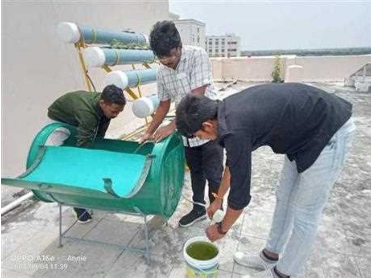
Fig 3:- collection of water sample for ammonia test by using siphoning pipe
